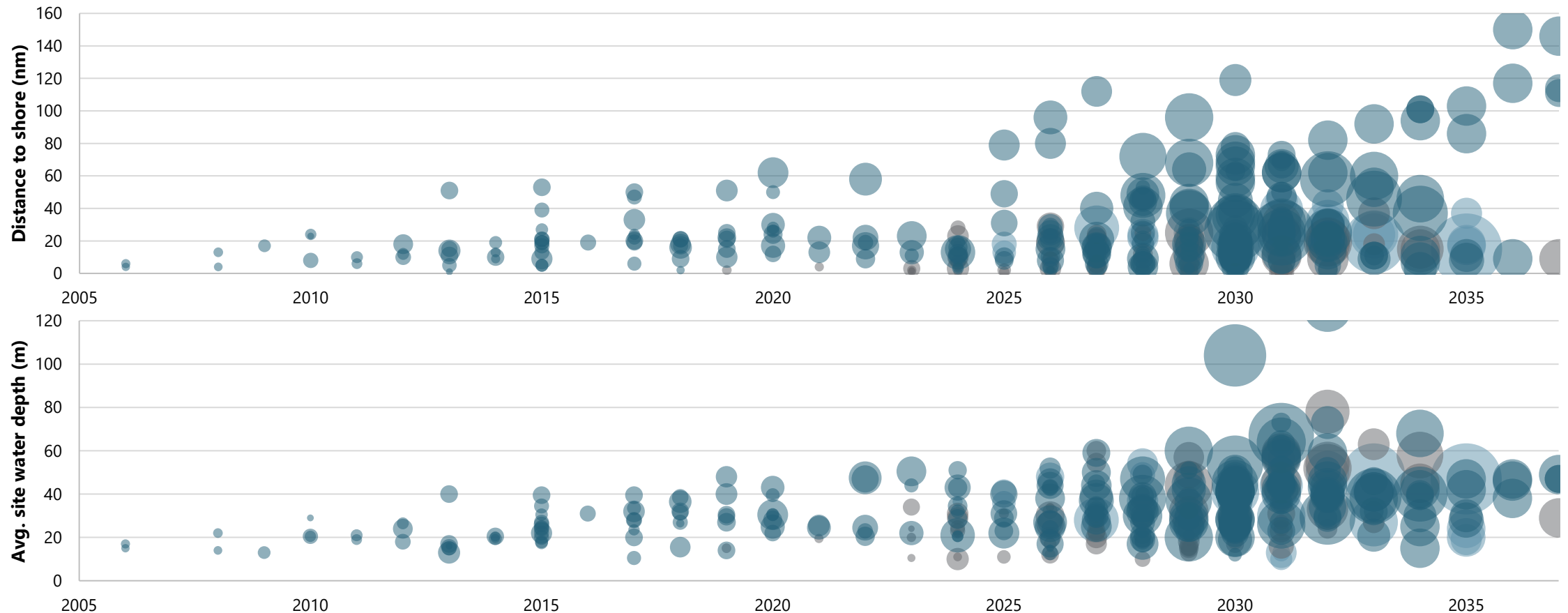
Distance to shore and average water depth of fixed bottom wind farms
